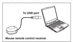
The remote control may fail to operate if the mouse remote control receiver is exposed to bright sunlight or fluorescent lighting.
