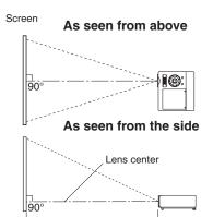
a (min length) = 0.0335 x Projection size (inches) - 0.05 a (max length) = 0.0402 x Projection size (inches) - 0.0488
