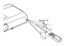
When operating the remote control from behind the projector, the infrared signal is reflected on the projecting surface and may travel a shorter distance to reach the projector depending on the shape and material of the projecting surface.
